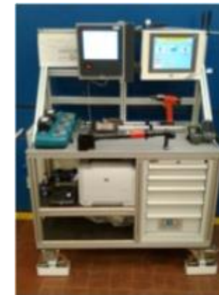
Example- Maserati Maserati FMS bench for Production w/battery & cable power tools + Tq. wrenches
