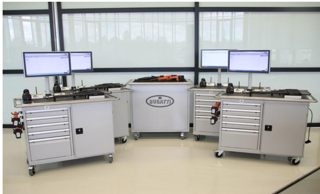
Example- Bugatti Bugatti w/Tq. wrenches & Smart Battery Tools for Production.
