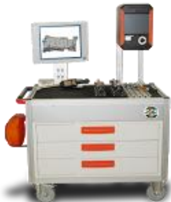
Example - FCA FCA FMS rework bench w/Tq. wrenches
